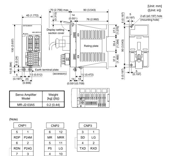
Note: One connector (5557-08R) and 10 terminals (5556) for CNP1 wiring are included in the package.
